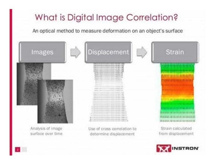
Optical methods have revolutionized the field of experimental research, providing accurate and non-contact measurement techniques for various applications. One notable advancement in this domain is the utilization of digital image correlation (DIC) for analyzing deformation and strain in materials. DIC combined with optical methods has opened up new possibilities in measuring complex phenomena with high precision and reliability.
