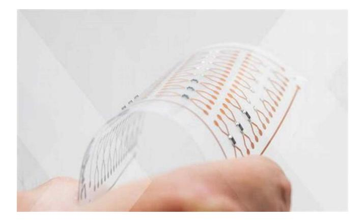
Flexible electronics is an emerging field that aims to create electronic devices that can be bent, rolled, or folded without compromising their functionality. This field heavily relies on novel materials that can withstand mechanical stress, such as flexible polymers and metal oxides.
