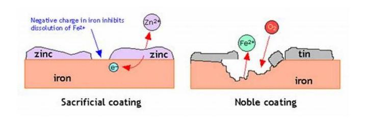
Corrosion is a natural process that affects various metals, but zinc possesses unique properties that make it a standout performer against environmental degradation. Zinc, in its pure form, showcases excellent corrosion resistance, rendering it highly valuable across numerous applications.
