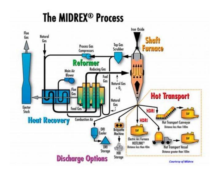
Sponge iron, also known as direct reduced iron (DRI), is a highly efficient and cost-effective alternative to traditional iron production methods. It is produced by reducing iron oxide (typically in the form of pellets or lump ore) using a reducing gas such as hydrogen or carbon monoxide. This article delves into the fascinating world of sponge iron production, exploring its benefits, the step-by-step process, and its applications in various industries.
