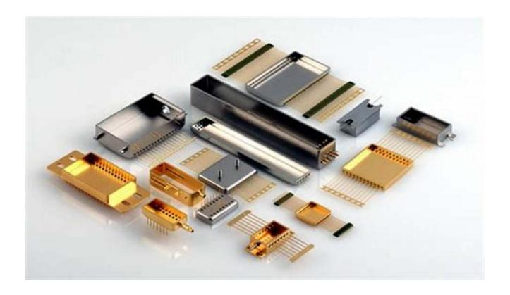
Metals, especially alloys, are extensively utilized in electronic packaging materials due to their excellent electrical conductivity, good thermal conductivity, and high mechanical strength. Aluminum, copper, and gold are commonly used metals in electronic packaging.
